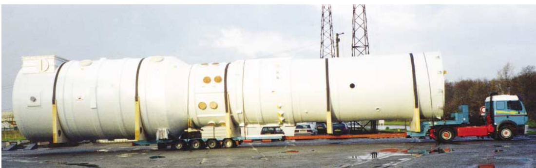
This FRP scrubber fabricated by Carlier Plastiques is among the tallest in the world – standing 31 meters high with sectional diameters of six and 4.5 meters.
